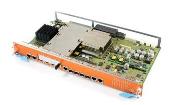
The central blade is the Ethernet switch and management blade for SI3000 Lumia 3.0. With its advanced Carrier Class network functionalities and various types of uplink interfaces it is an Ethernet switch and aggregation platform for subscriber blades and external network elements. Two central switch blades in MEC are logically seen as one device, which offers both extremely high bandwidths (40G/slot) and flexibility in building various network topologies like subtending or Ethernet rings.
